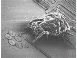
A <u>mite</u> next to a <u>gear</u> set produced using <u>MEMS</u>. Courtesy Sandia National Laboratories, SUMMiTTM Technologies, www.mems.sandia.gov.
